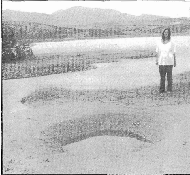
Plate 3: Sand boil and crater on south-eastern banks of Polifiton Reservoir.
